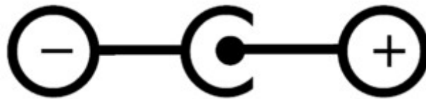
Drawing 1: Power Jack polarity
